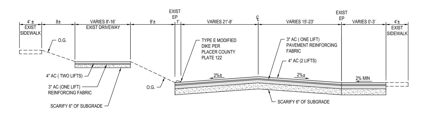
CULVER STREET TYPICAL SECTION - STA 12+57 TO 13+80
