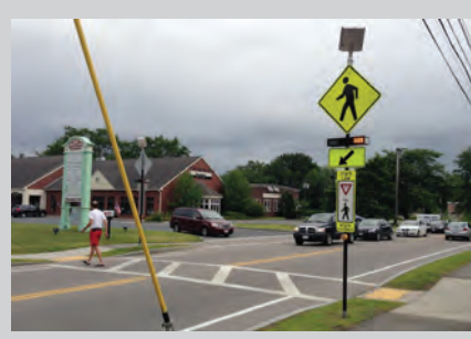
Rectangular Rapid Flashing Beacon (RRFB)
