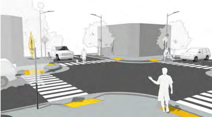
Curb ramps and crosswalk
