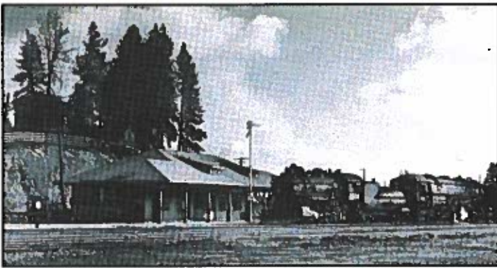
In this photo from the early 1940's, an eastbound Southern Pacific cab-forward locomotive pauses in front of the Colfax Passenger Depot. A Colfax-based helper locomotive has been added in front of the big cab-forward. The helper will provide added power for the heavy grades between Colfax and Emigrant Gap.
