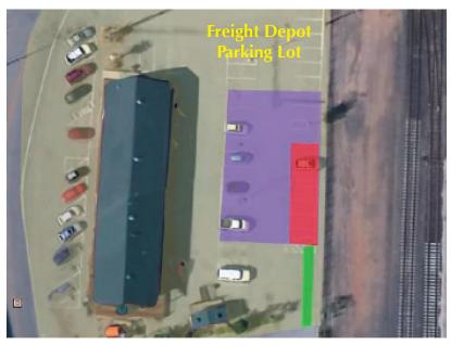
Proposed site of Colfax Microgrid installation. The purple area will be parking area for generators. The red and green areas will be for distribution and transformer equipment.
